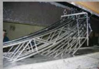
Trusses being hot dip galvanized.
